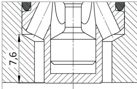
The nose of the valve protrudes by 7,6mm into ID 12mm of the cavity.
