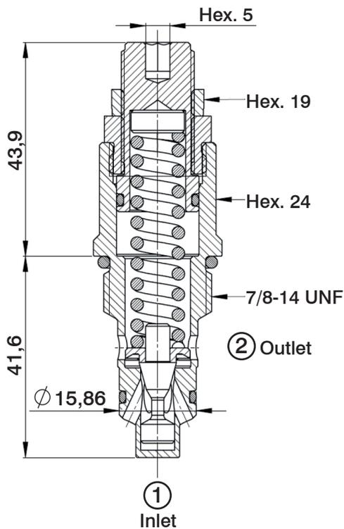
To secure the setting, torque the Hex19 nut with 25-30 Nm
